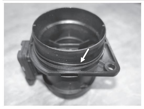
3) Install the thinner, supplied o-ring around the base of the inlet of the MAF sensor.
