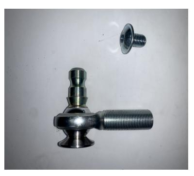
**Step D**Apply half packet of anti-seize to spherical heim joint
