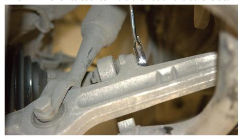
**Step 4**Remove the factory front sway bar end links.
