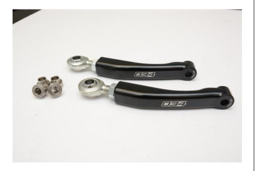
You are now ready to start the installation process. Use the length of the stock component as a starting point for the length of the 034 adjustable end links; expand or compress as best fits your needs
