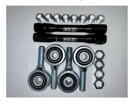
**Step B**Apply half packet of anti-seize to Density bushing
