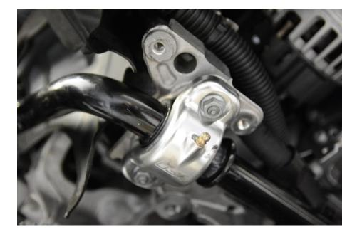
**Tip:** Orient brackets with zerk fittings facing forward for easy greasing.
