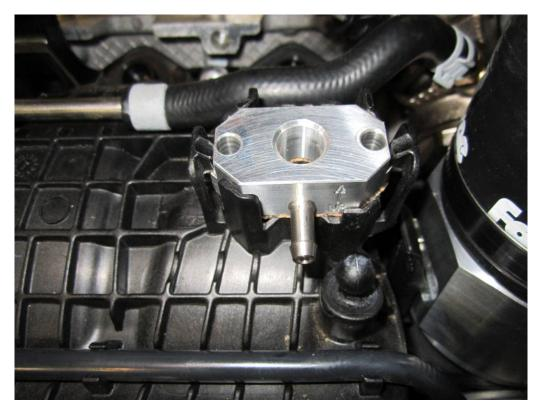
3. Now fit the sensor to the boost tap block using the posi screws provided and tighten with a posi drive screwdriver.
