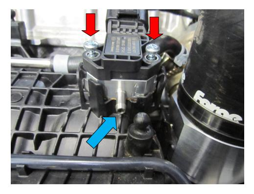
4. Now fit the vacuum pipe to the nipple arrowed blue in the picture above and route to the required location .
