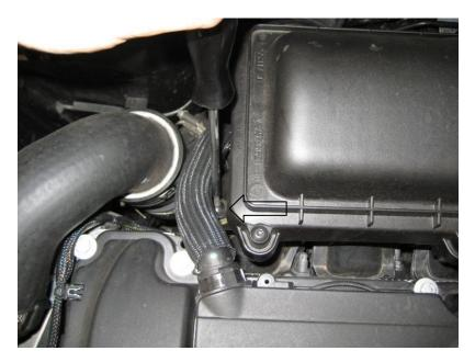
Remove the MAP sensor from the top of the inlet manifold as shown, then push it firmly into the supplied Forge MAP sensor boss. A little silicon spray will make it easier. You can then attach the hose from your boost gauge to the takeoff on the block, then reattach the whole assembly back to the inlet manifold with the screw provided, and refit the airbox and hoses removed
