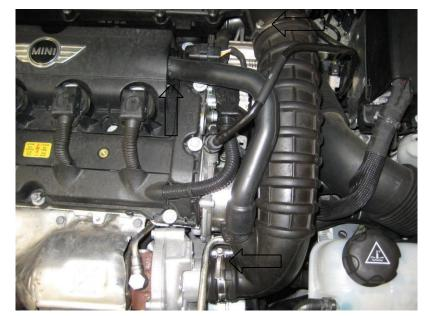
Lift the bonnet and begin by undoing the two jubilee clips holding the hose between the airbox and turbo inlet. Pull off the breather to the cam cover and remove the whole hose assembly from the car.
