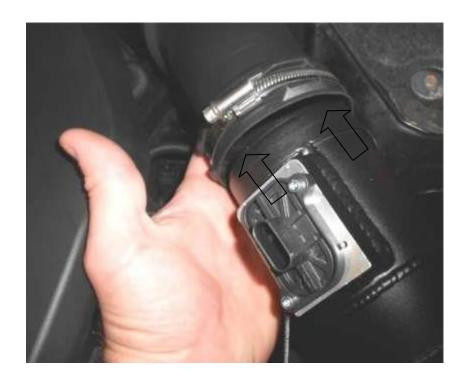
14. Using a 7mm hose clamp driver tighten the hose clamp.
