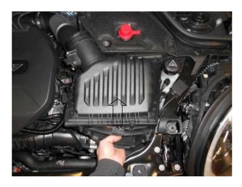
7. Using a T20 Torx driver undo the 2x screws and carefully remove the MAF sensor. Handle with care.
