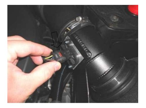
16. Refit the OEM ducting, using a 10mm socket secure with 2x nuts.
