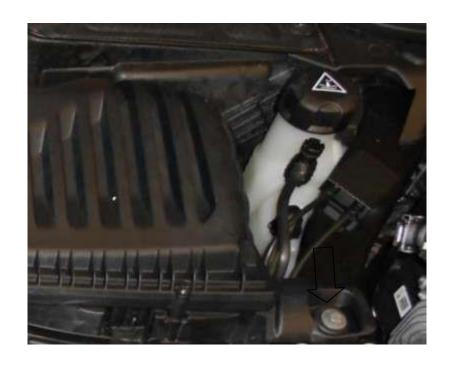
6. Pull the intake pipe off of airbox pipework and firmly pull the airbox upward to release it.
