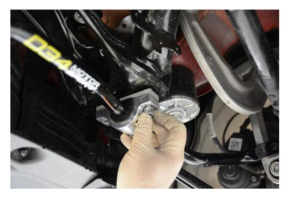
**Step 8** – Attach the sway bar end links to the 034Motorsport Dynamic+ Adjustable Rear Sway Bar using the factory hardware. Torque to 40 Nm + 180 Degrees.
