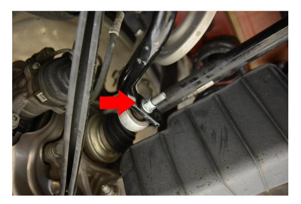
**Step 9** – Tighten the sway bar mount bracket bolts to 28 Nm.
