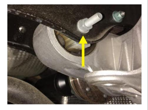
**Please Note:** We recommend replacing this bolt after removing. The part number for factory bolt is N10771601.
