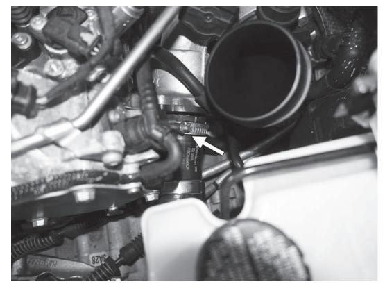
15) On the turbocharger outlet, loosen the 7mm hose clamp on the outlet hose, and remove the hose from the turbocharger.
