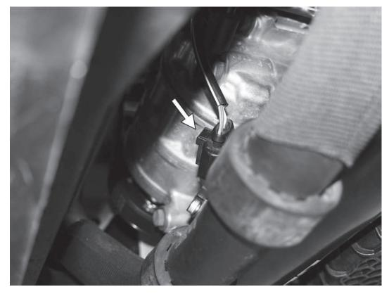
45) Reconnect the electrical connector from the wiring harness to the MAP sensor.
