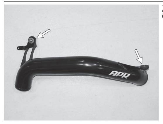
17) Install the two rubber grommets and screws onto the APR turbo outlet pipe as shown.
