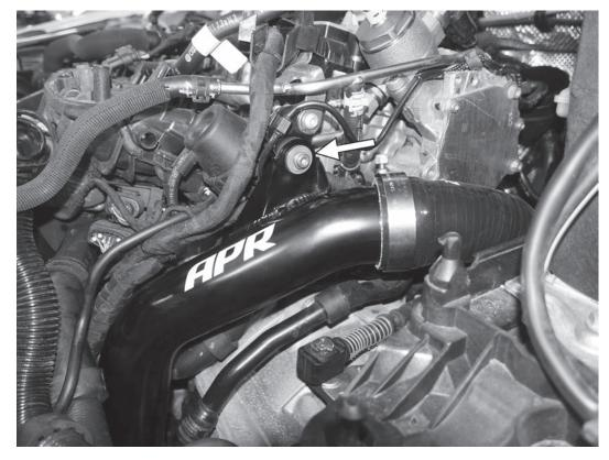
25) Install the factory T30 screw with the rubber grommet to the original stock pipe mounting point on the top of the engine. Torque the screw to 62 in-lbs (7Nm),
