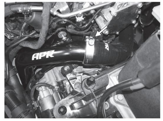
23) Install the upper side of the APR outlet pipe to the APR silicone hose with the 2.75" (-0275) hose clamp. Orient the hose clamp so it can easily be tightened, but leave the clamp loose for now.
