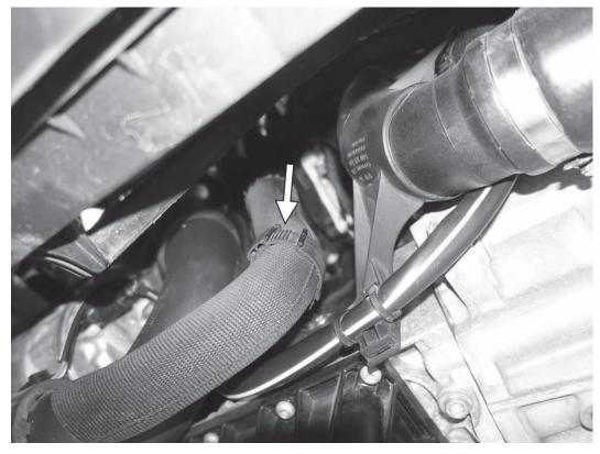
3) From underneath the car, disconnect the hose from the clip that connects the coolant hose to the front of the engine. Separate the clip from the hose, and then remove the clip from its mounting tab.
