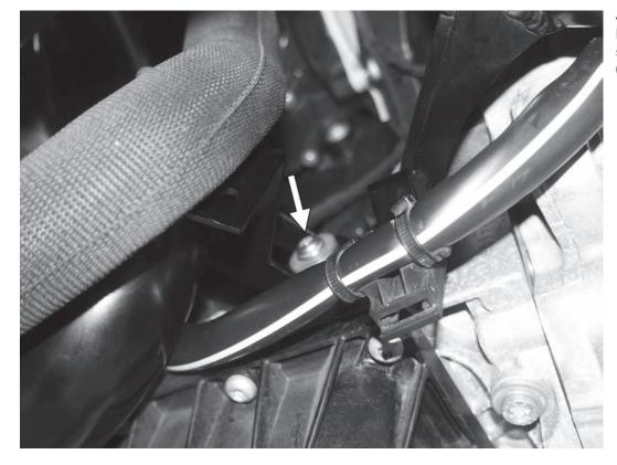
43) Secure the APR intercooler pipe by installing the T30 screw on the left side of the pipe. Torque the screw to 62 in-lbs (7Nm).
